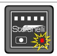
B. **the engine is running on LPG** (with the petrol LED off and the fuel level LED on)
